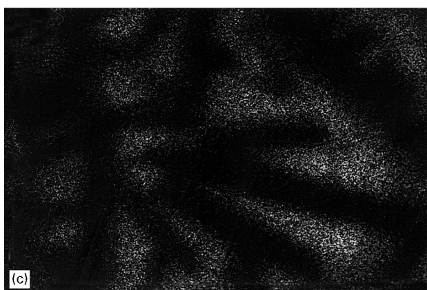
Figure 3 (a) Scanning electron micrograph and (b–d) EPMA photographs of the polished surface in the 50 mass % mullite/50 mass % \text{Cr}_2\text{O}_3 compact heated in a carbon powder bed at 1500 °C for 2 h (b) Cr, (c) Si, (d) Al.
