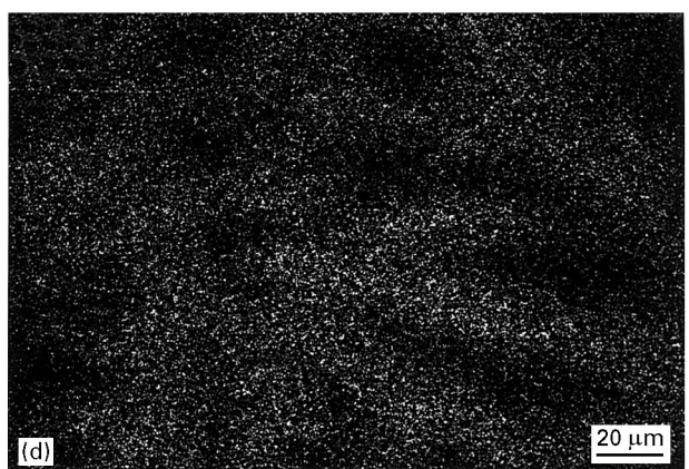
Figure 3 (a) Scanning electron micrograph and (b–d) EPMA photographs of the polished surface in the 50 mass % mullite/50 mass % \text{Cr}_2\text{O}_3 compact heated in a carbon powder bed at 1500 °C for 2 h (b) Cr, (c) Si, (d) Al.
